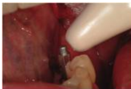
Figure 2. Magnetic transducer attached to one implant with probe in close proximity taking the resonance frequency measurement.
