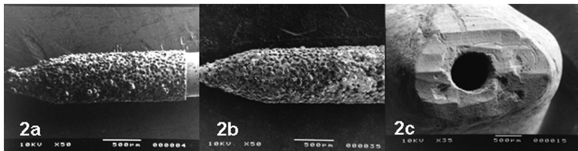
Figure 2. Trinity tip: (A) before utilization; (B) after utilization; (C) preparation with tips.
