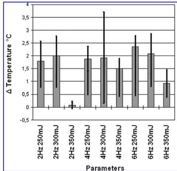
FIG. 3. Temperature increases without spray (means and standard deviations).
