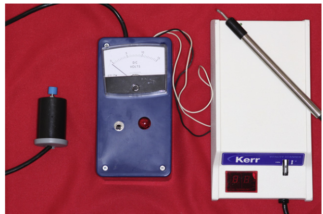
Figure 1. The experimenter's box is shown in the middle. The modified electric pulp tester (right) is shown along with the hand-held push button device (left) used to control the current output of the pulp tester.
