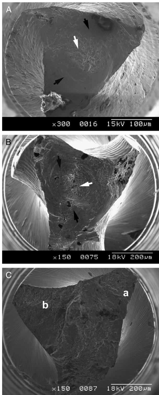
**Figure 1.** Fractographic analysis of rotary NiTi instruments. For overloading fractures of TF (A) and PF (B) samples, peripheral smooth (black arrows) and central dimpled (white arrow) areas are visible. For fatigue failures of PF samples (C), multiple striations (a) and surface pattern with dimples and cones (b) are observed in the same fracture plane.
