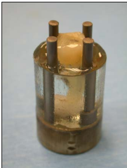
Figure 2b. Muffle device with Teflon sleeve removed.
