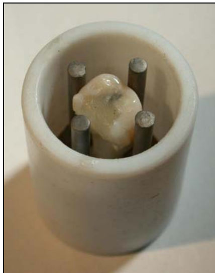
Figure 2b. Muffle device with Teflon sleeve removed.
