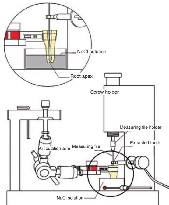
Figure 1 Measuring unit.
