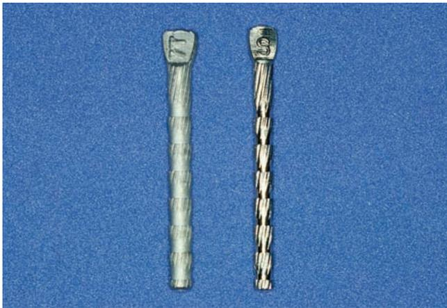
FIG 5. A titanium alloy post (left) and a stainless-steel post.
