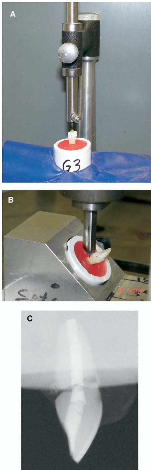
**Figure 1.** (A) Mounting tooth perpendicular to the acrylic resin utilizing a surveyor. (B) Chisel shaped Instron tip positioned at lingual CEJ before fracture. Note: 130 degree angle to long access of the tooth. (C) Tooth fracture through cervical root structure and root canal filling material.
