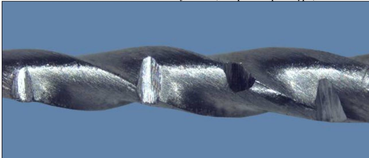
*File with notches that transverse a spiral (McSpadden prototype)*
