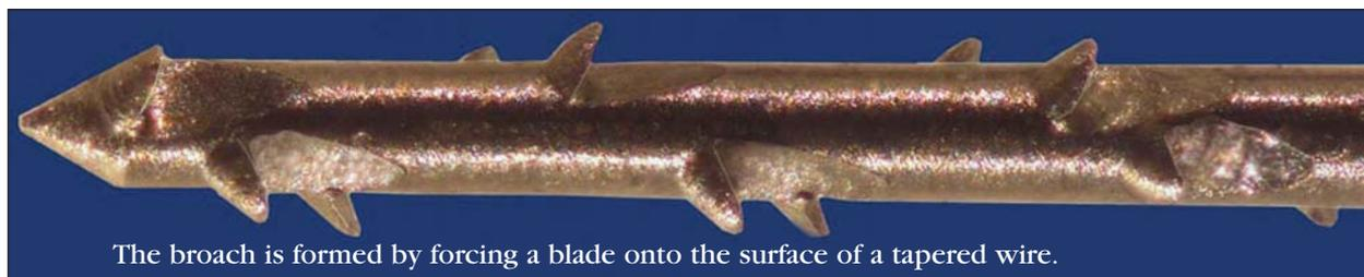
The broach is formed by forcing a blade onto the surface of a tapered wire.
