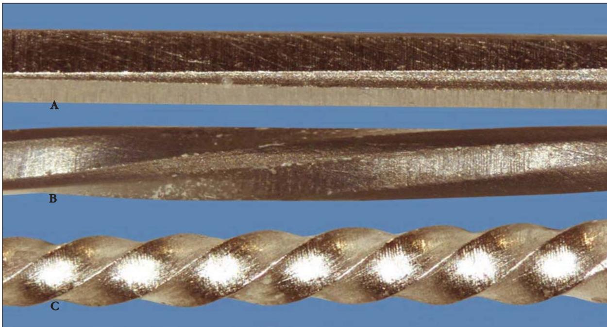
Fig. 2 A. A tapered pyramidal wire is used as a blank for forming a file.
