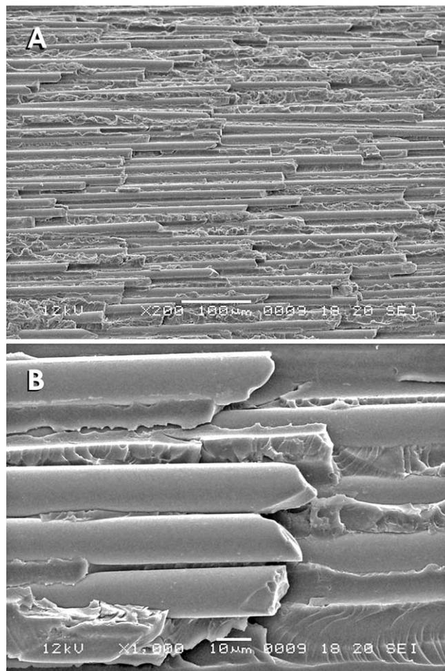
**Figure 1.** Representative SEM micrographs of a post surface after etching with 10% hydrogen peroxide for 20 min. (A) At a low magnification, exposure of the quartz fibers could be seen, as a result of the dissolution of the surface epoxy resin. (B) A high magnification view of the exposed quartz fibers, showing that they were not damaged by the etching treatment. Similar results were achieved when etching was performed with 24% hydrogen peroxide for 10 min (not shown).
