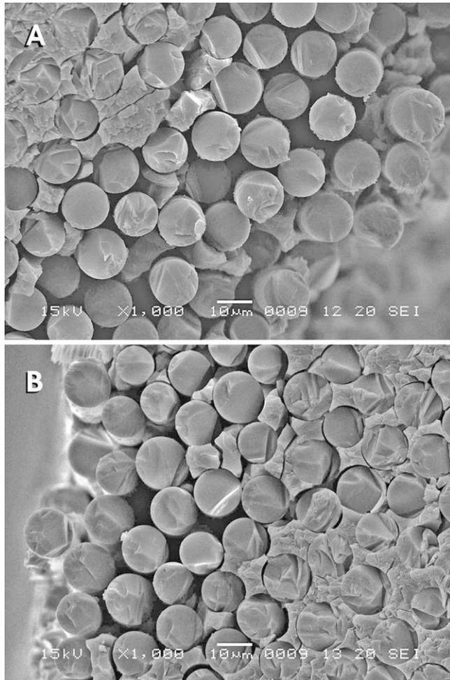
**Figure 2.** SEM images of the cross sections of fiber posts after treatment with 24% hydrogen peroxide for 10 min (A) and 10% hydrogen peroxide for 20 min (B). Dissolution of the epoxy resin from the post surfaces exposed the quartz fibers to a depth of 50 μm for silanization as well as created additional spaces for micromechanical retention of the flowable composites.
